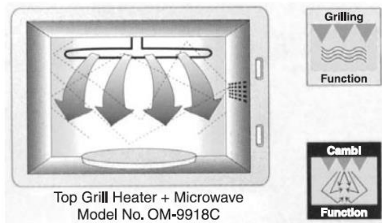
Fig. 1.7 In combo mode of cooking, the microwave along with the grill can be used simultaneously to cook faster for perfect browning and crispy texture.
